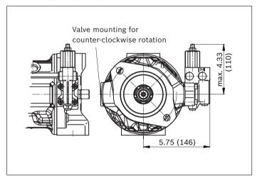
**▼ DRG - Pressure controller, remotely controlled**
