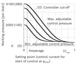
► Hysteresis static current-pressure characteristic curve < 45 psi (3 bar).
