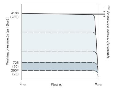
Characteristic curve valid at n<sub>1</sub> = 1500 rpm and  $\vartheta_{\text{fluid}}$  = 122 °F (50 °C).
