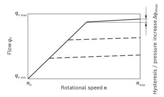
Characteristic curves valid at  $n_1$  = 1500 rpm and  $\theta_{fluid}$  = 122 °F (50 °C).
