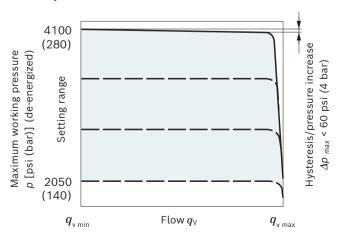
Characteristic curves valid at  $n_1$  = 1500 rpm and  $\vartheta_{fluid}$  = 122 °F (50 °C).
