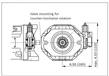
**▼** DRG - Pressure controller, remotely controlled
