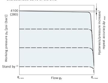
Characteristic curve valid at  $n_1$  = 1500 rpm and  $\theta_{fluid}$  = 122 °F (50 °C).
