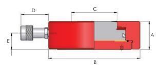
Note: All models, excluding HVL100, are fitted with extension nipple for required coupling clearance (drawing is without coupling extension nipple).
